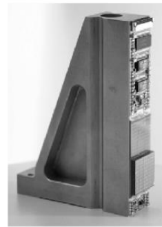
CT Detector module based on integrated CMOS photodiodes
